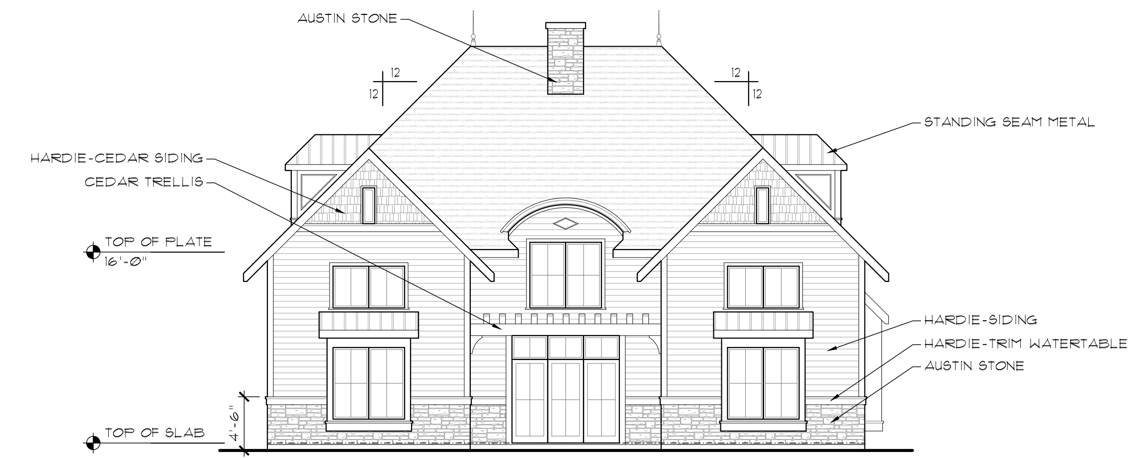
PROPOSED WEST ELEVATION SCALE - 1/8" = 1'-0"
