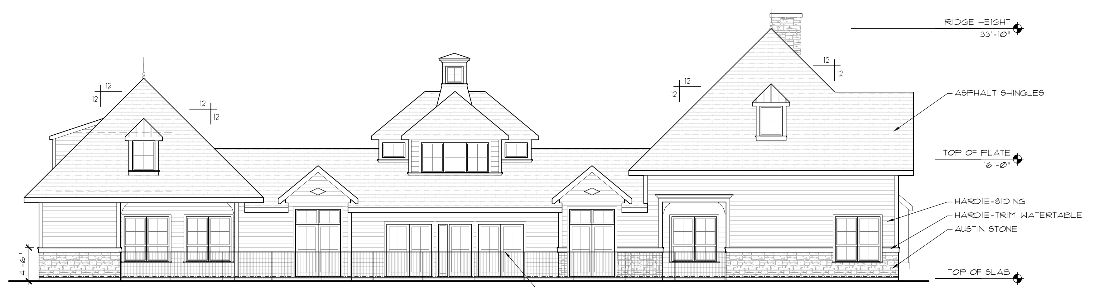
PROPOSED NORTH ELEVATION SCALE - 1/8" = 1'-0"
