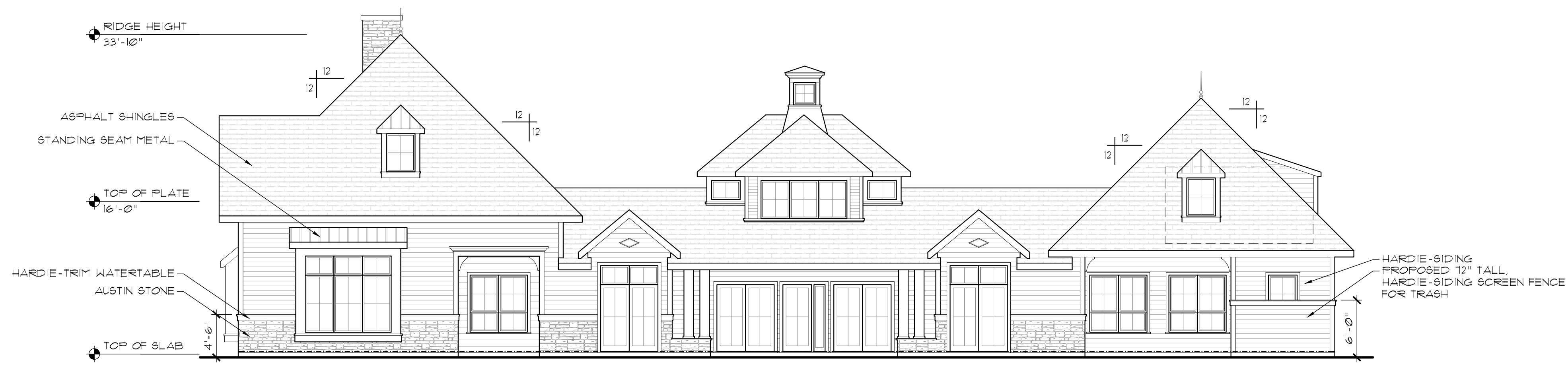
PROPOSED SOUTH ELEVATION SCALE - 1/8" = 1'-0"
