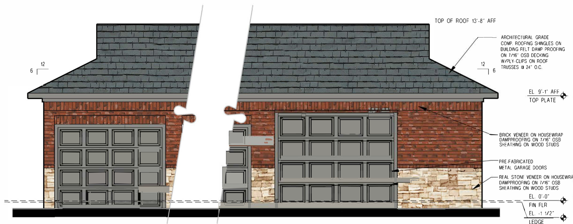
16 Detached Garage Elevation - With HC Bay SCALE: 3/8" = 1'-0"
