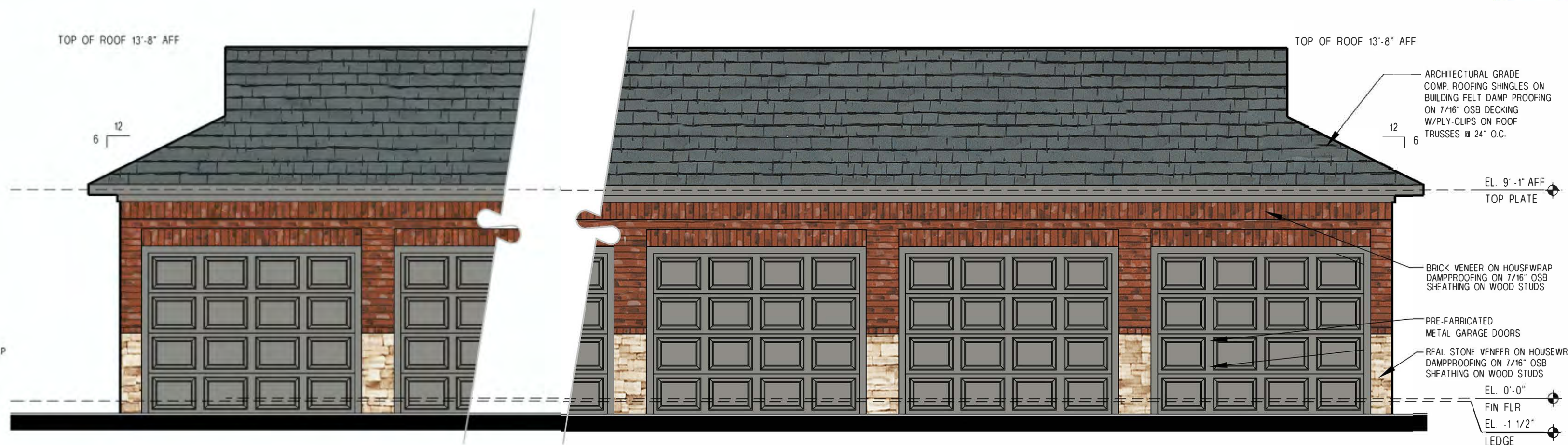
13 Detached Garage Elevation SCALE: 3/8" = 1'-0"
